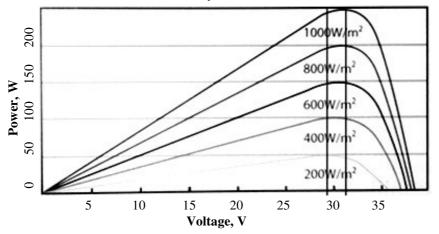
Fig. 2. Power-voltage curve of PV panel (Producer's information)
