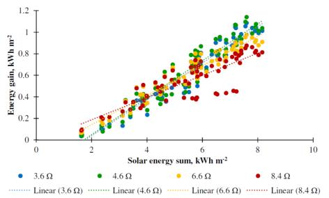
Fig. 4. Dependence of energy gain from PV panel with several load resistances on solar irradiance
