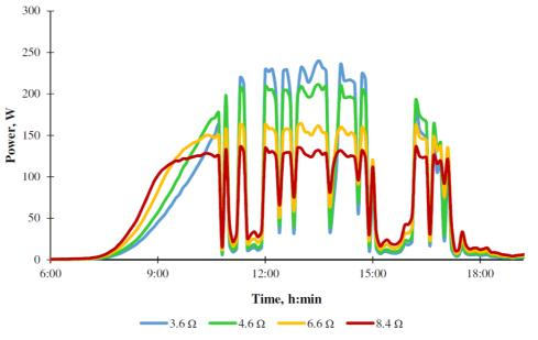
Fig. 3. Daily course of power produced by PV panels with different load resistances (11 of July, 2018)
